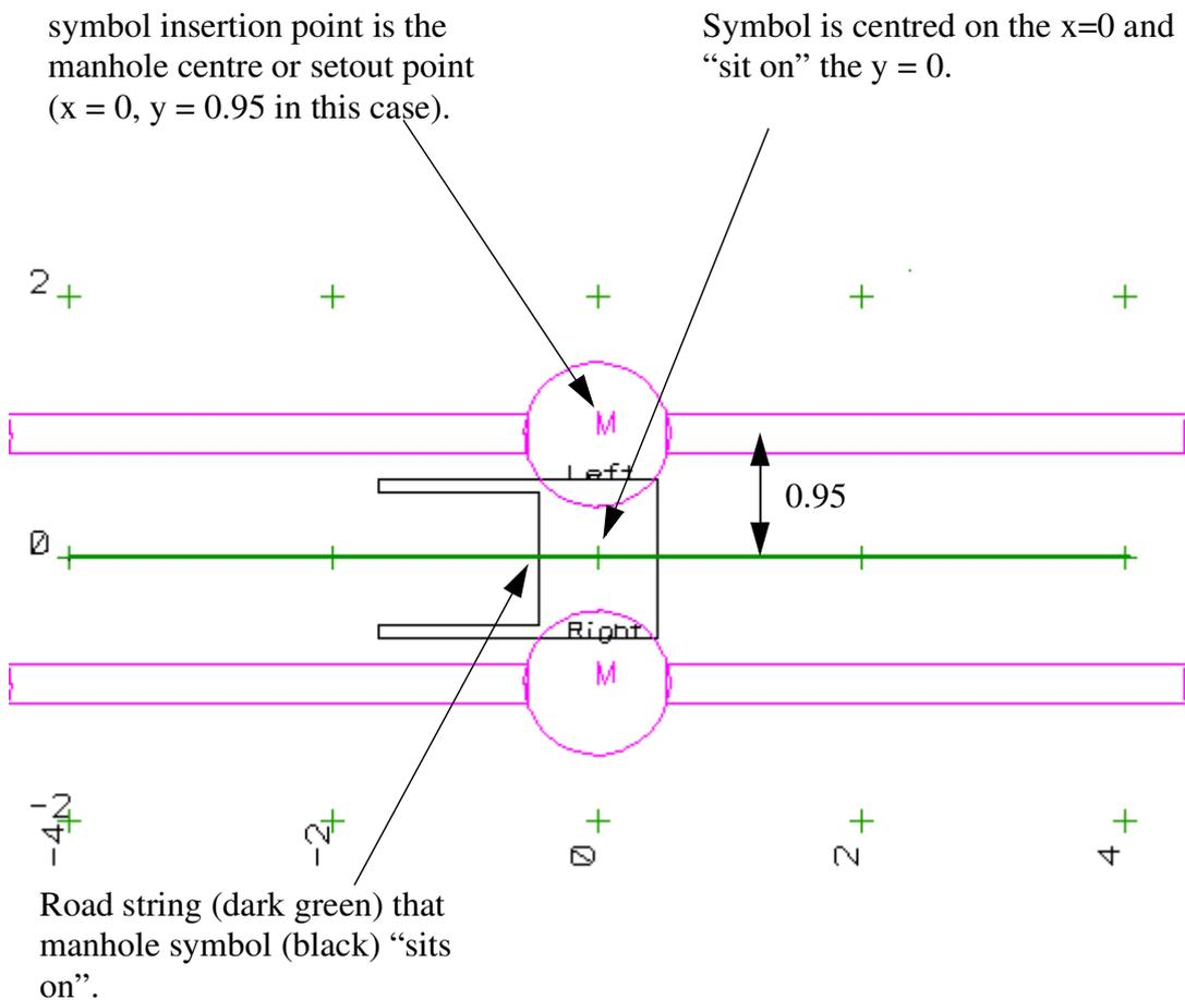
To create the symbol in 12d draw the left pit symbol in a model by itself. The pit should “sit on” the zero “y” grid line. A 900 wide by 600 long inlet with a 1.2m lintel is shown above.
