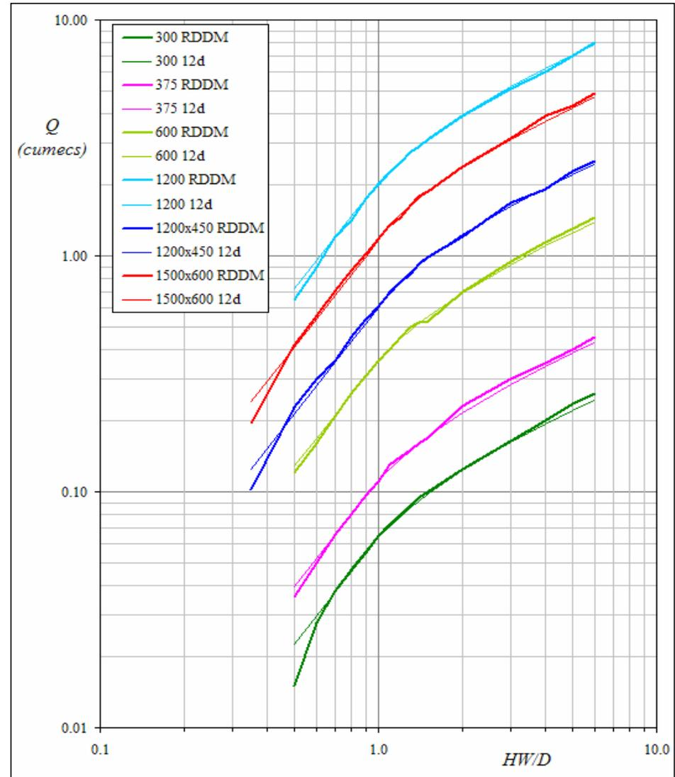
Comparison between results from RDDM headwater nomographs and 12d Model formulae, for several standard pipe and box culvert sizes (in millimetres)
