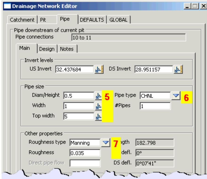
5. Set the **Height**, **Top width** and **Bottom width** of the channel.
