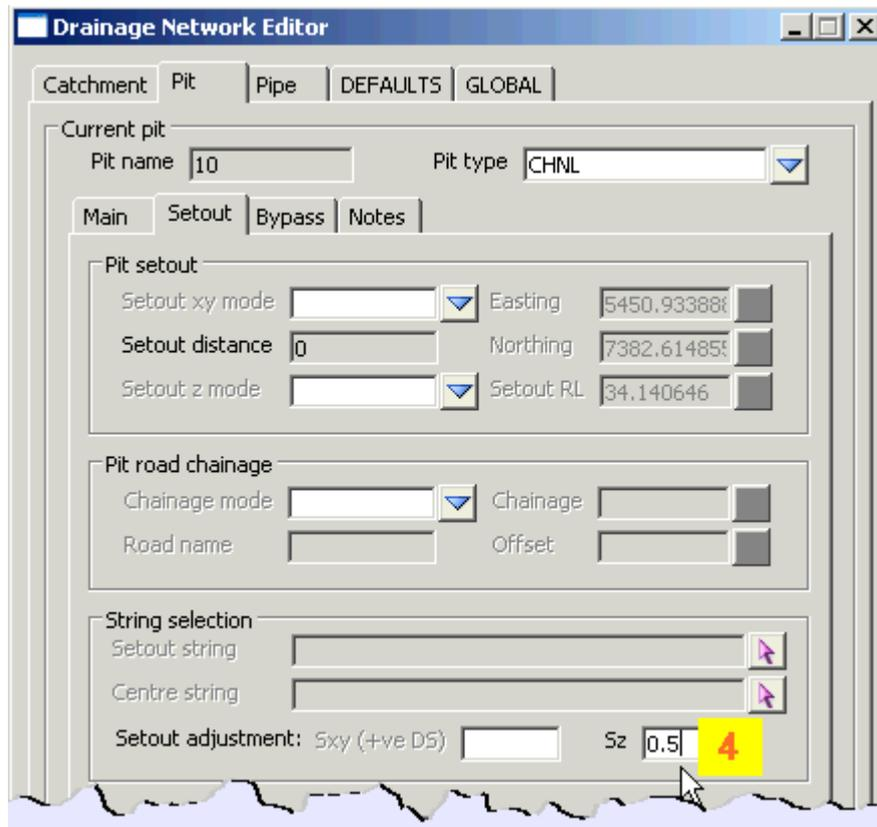
4. Enter the Sz equal to the height of the channel. This will set the grate level at the top of the channel.
