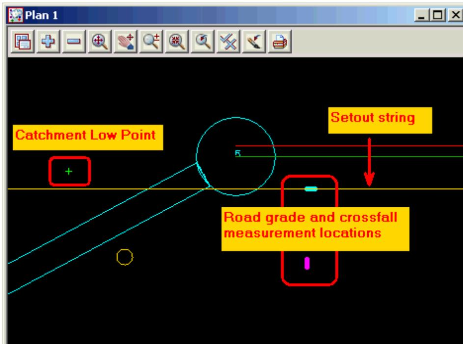
The green line indicates where road grade was measured and the magenta line indicates where the road cross fall was measured.
