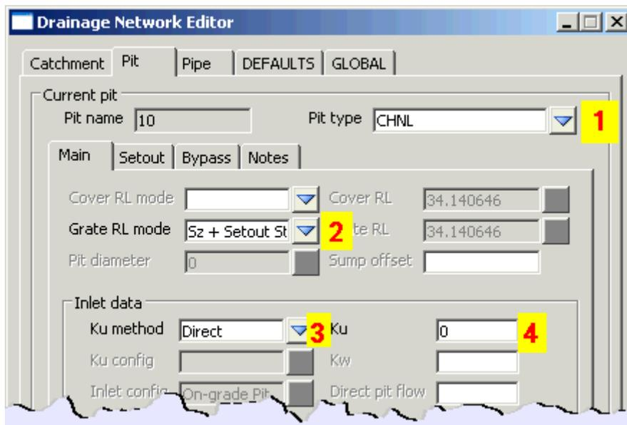
1. The **CHNL** pit type has a 200% inlet capacity and a diameter of zero. This will result in a single line on the drainage long sections instead of a pit.
